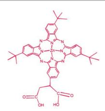
**Pushing and pulling** by three *tert*-butyl and two carboxylic acid groups, respectively, results in a sensitizer (see picture) that exhibits an incident photon-to-current conversion efficiency of 75 %. A cell sensitized with this compound gives a short-circuit photocurrent density of  $(6.50\pm0.20)~\text{mA}~\text{cm}^{-2}$ , an open-circuit voltage of  $(635\pm30)~\text{mV}$ , and a fill factor of  $0.74\pm0.03$ , which corresponds to an overall conversion efficiency of  $3.05\,\%$ .
