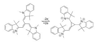
The Y-shaped  $\pi$  systems in trinuclear cyanines can, through a formal two-electron transfer, form a core methylenecy-clopropane unit with three shorter, isolated  $\pi$  systems (see picture). Studies of
