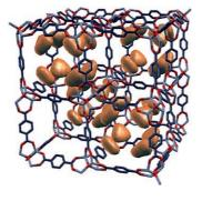
Doing the locomotion: When benzene molecules diffuse through the metal organic framework MOF-5, they accumulate in pockets (see picture). Molecular dynamics simulations reveal that the correlated lattice motion increases this binding. Only when the lattice dynamics are considered in the simulation, can the experimental diffusion constants be reproduced.
